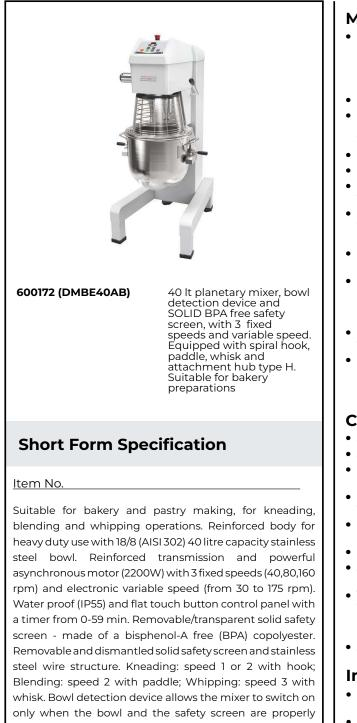
installed and positioned together. Equipped with accessory drive hub type H (accessories are not included). Supplied with 3 tools: spiral hook, paddle and reinforced whisk.
